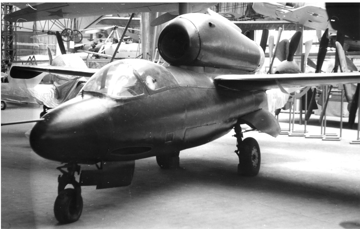
The machine with its museum paintwork scheme / The position of the Pitot tube TT , located on the nacelle during French testing is unusual. The original German Pitot tube is missing completely.
